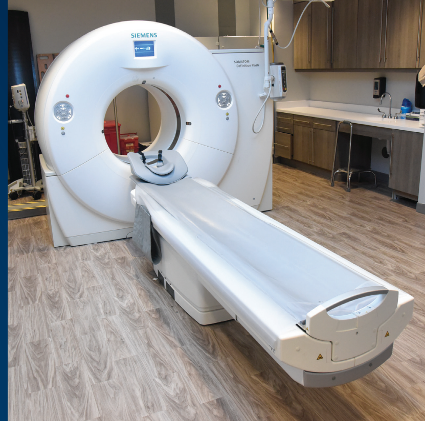
The dual-source CT scanner, complete with Stellar Detector, allows faster acquisition of images at minimal radiation dose without compromising image quality.
